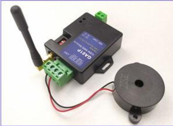
Before testing a new device, you must first confirm whether your device is 2G, 3G, or 4G. Need to prepare a SIM card. Then insert the SIM card, and judge whether it is connected to the Internet according to the status of the LED after power on.
